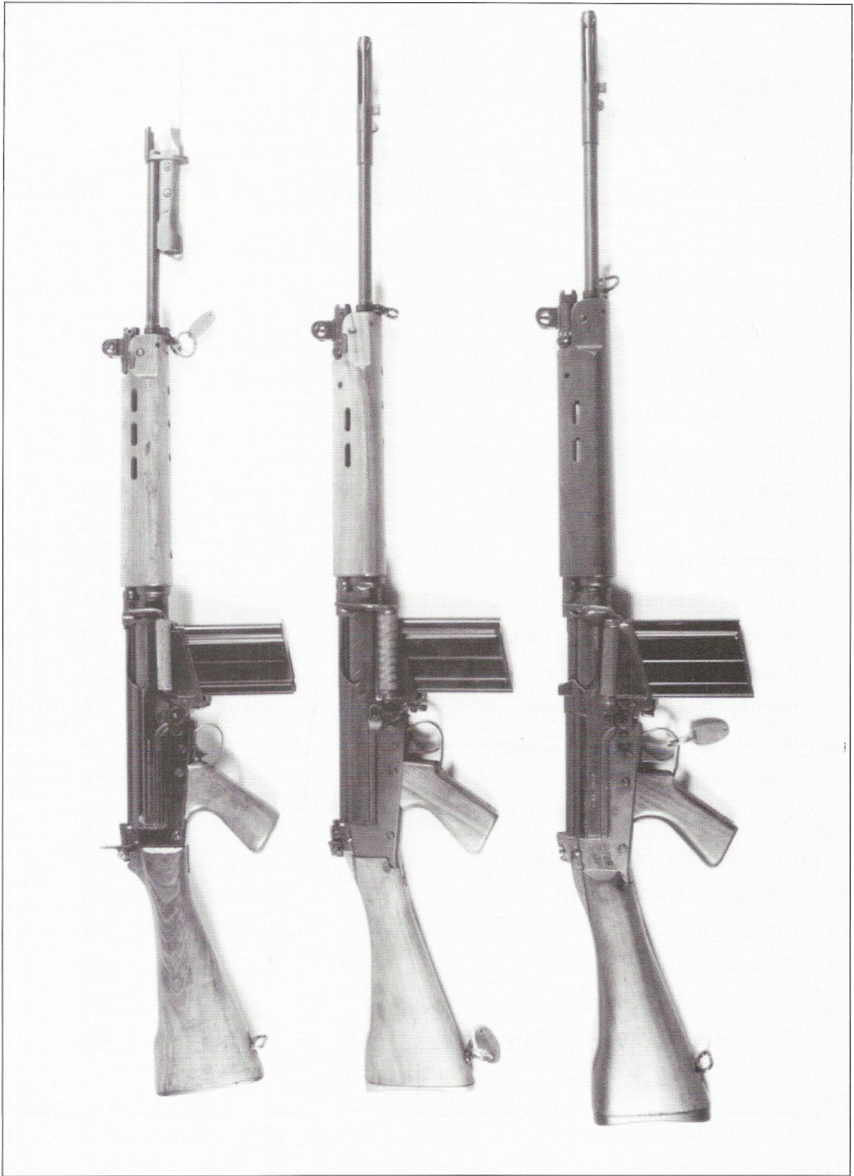
From left— F.N. made X8E1 trials rifle, early Enfield production L1A1 rifle and Canadian C1 production at Long Branch. Note the different dustcover, backsight and carry handle on the C1. M.O.D. Pattern Room
