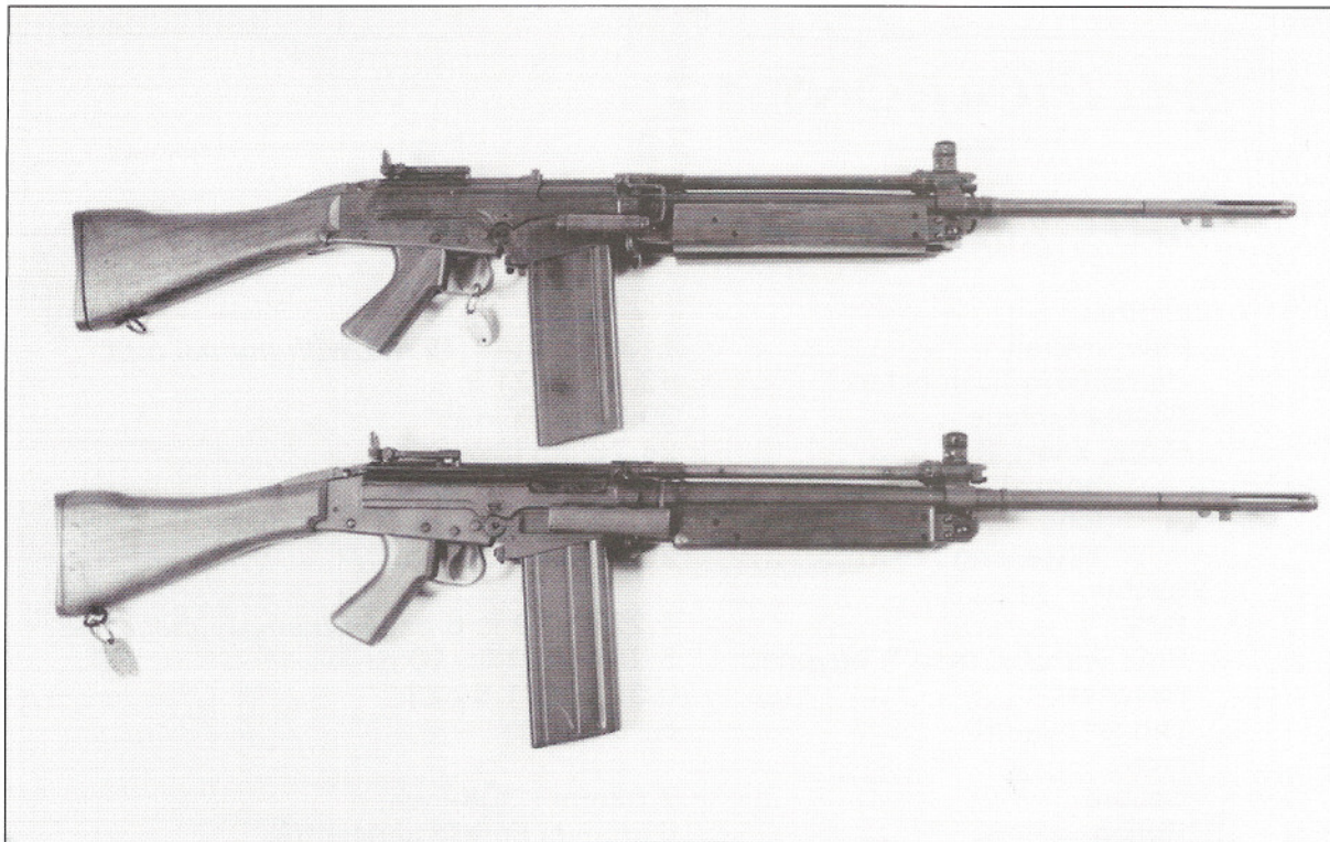
Canadian C2 at top compared with Lithgow L2A1 rifle below. The tangent rear sight originated in Canada. Note the different auto rifle carry handle, allowing for the different centre of gravity. M.O.D. Pattern Room
